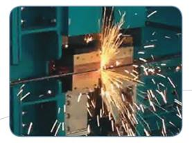
By this EVO control package installed on the STI welders, customers are able to program in details all variables and to detect and see in real time the applied forces, heat and speed variations, as well as to save data for certifications of the products.
