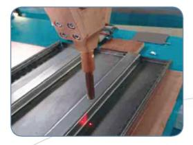
In the attached picture, it is possible to see a welding head of a "ROOF" model, the most flexible solution for assembly and manufacturing metallic doors and cabinets of any kind, available as well in its automatic version "ROBOSIDE".
